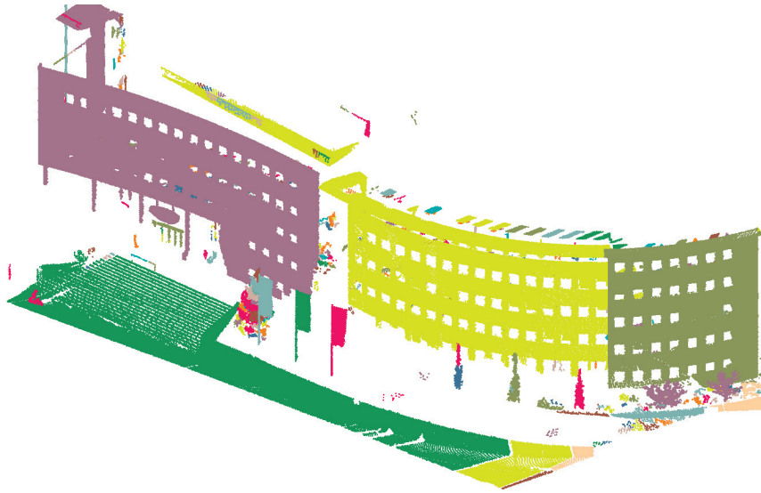
Figure 3.6: Segmentation with the smooth surface method.
