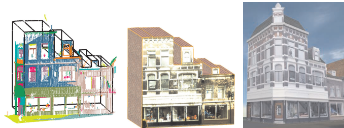
Figure 7.22: Reconstruction of Markt 60 right facade (left: geometry model; middle: textured model; right: by traditional approach)
