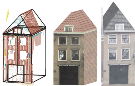
Figure 7.19: Reconstruction of Markt 49 (left: geometry model; middle: textured model; right: by traditional approach)
