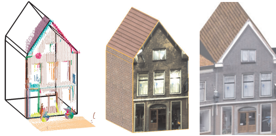
Figure 7.20: Reconstruction of Markt 57 (left: geometry model; middle: textured model; right: by traditional approach)
