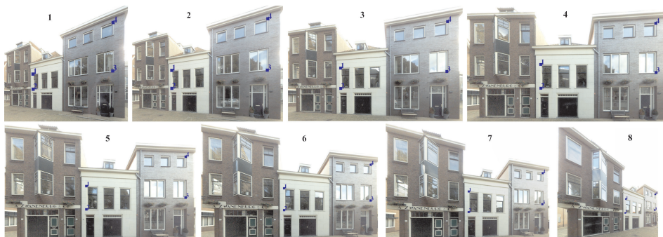
Figure 5.7: Locating occurrences of the same laser points in different image perspectives.
