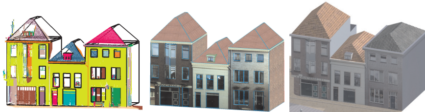
Figure 7.14: Reconstruction of Markt 31-34 (left: geometry model; right: textured model; bottom: by traditional approach)
