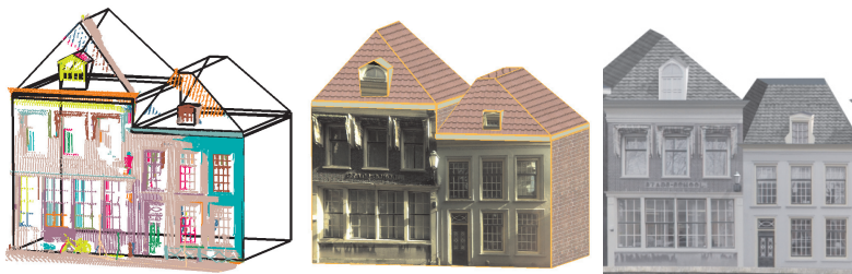
Figure 7.16: Reconstruction of Markt 44-46 (left: geometry model; middle: textured model; right: by traditional approach)
